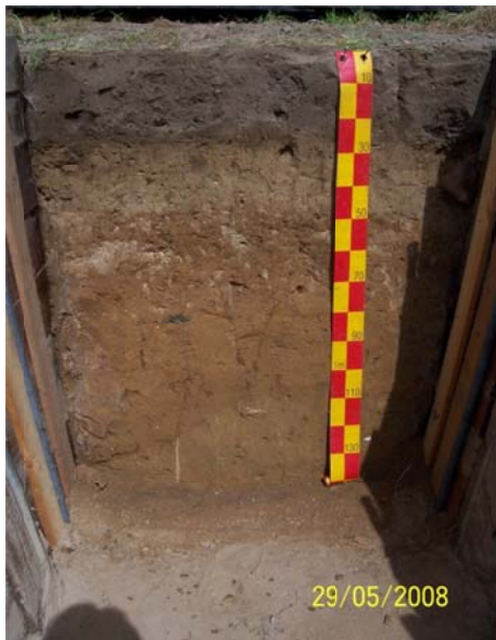
Albic Luvisol from sand overlaying loam and deep glacial till (37-43 soil points)
