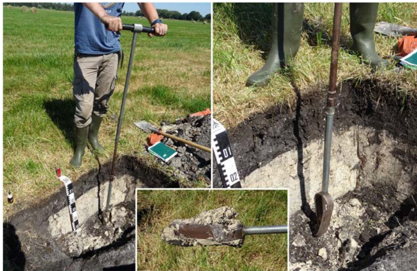
Figure 19: Use of an Edlmann drill
